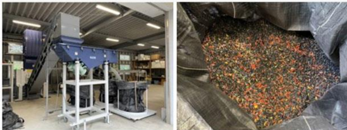
Converting hard drifting plastic into fuel chips from Elcom website
