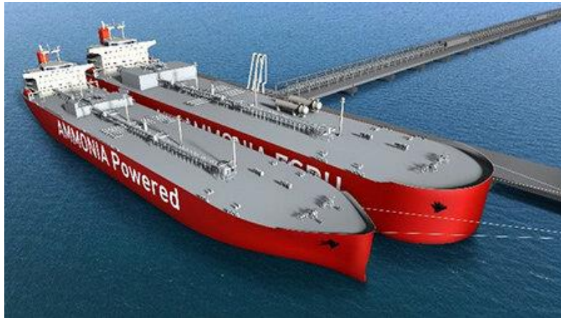
Ammonia transport vessel on the left and ammonia FSRU on the right From MOL website
